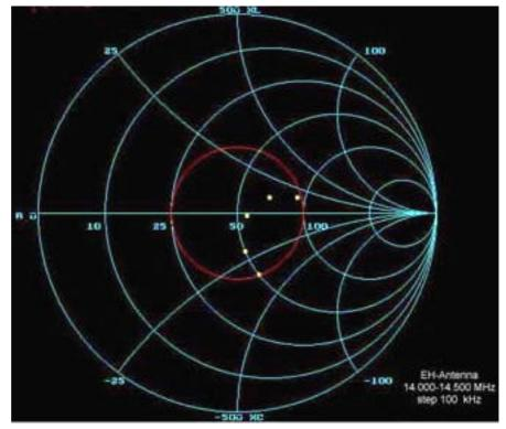
Input impedance of RH-ANT.#4 Red circle SWR=2:1 BW= 100 kHz @ SWR 2:1
