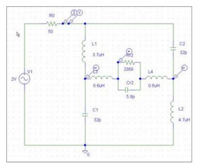
This is the diagram equivalent of #2 EH-Antenna.
