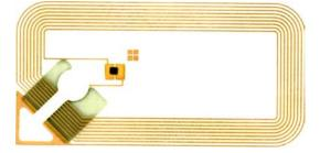
The tag is actually a full transponder, with the internal circuitry powered by the RF signal from an associated "reader". With the ability to interface the reader to a standard computer, and the ability to read or program the transponder from a distance, the applications for such a device are limited only by imagination.
